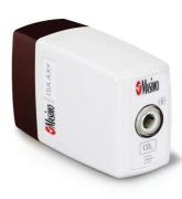
ISA AX+: Provides anaesthetic gas measurements in addition to capnography
