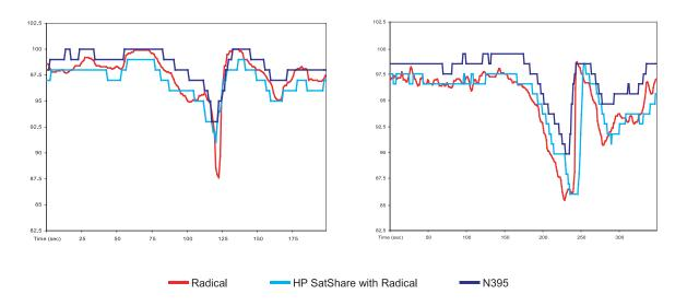
Further testing characterized the response times of the Radical, interfaced via SatShare, and the Nellcor N395, reporting a step change in saturation. The following chart shows the response time test results. From this table it is clear that, despite a slight delay in the overall response, Radical interfaced via SatShare still responds faster to changes in physiology than the Nellcor N395.
